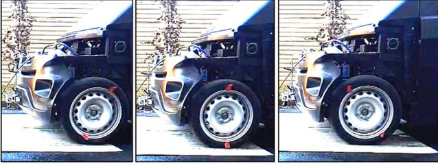
Fig. 16. Image sequence (from left to right) of the prototype EV with “Pre-NMPC with  $\tau_{hb}$ ”, during the same high-to-low tire-road friction step change test as in Fig. 14. The wheel does not tend to lock, and meets the soft constraint defined by the slip ratio threshold.
