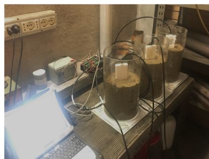
Figure 1. Experimental setup of the three mesocosms with the sensors for monitoring electrical conductivity and permittivity and the connection with the datalogger and the laptop.
