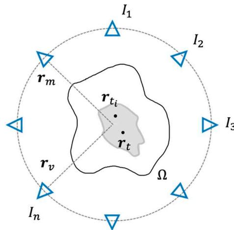
**Figure 2.** Schematic view of the phased antenna array surrounding the domain of interest  $\Omega$  and the target volume. Each antenna is indicated by a blue triangle, while the grey area represents the target volume.
