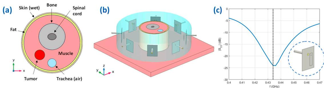
**Figure 3.** Simplified numerical testbed. (a) Top view on the plane  $z = z_t = -15$  mm of the simple neck model implemented in COMSOL, with the considered different tissues; (b) Geometry of the HTP applicator, the simplified neck, and the waterbolus; (c) Reflection coefficient of a single-feed patch antenna of the simulated array.
