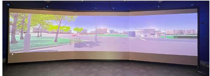
Figure 2 Immersive Reconfigurable Innovative System (IRIS) Cave platform in its open configuration displaying the Digital Twin model of Fuorigrotta, Naples, developed within MOST Project.
