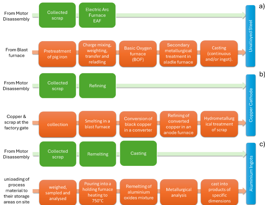
Figure 4.3 Manufacturing processes (dataset from Ecoinvent database) and recycle processes (energy requirements from the literature) for a) steel b) copper c) aluminium
