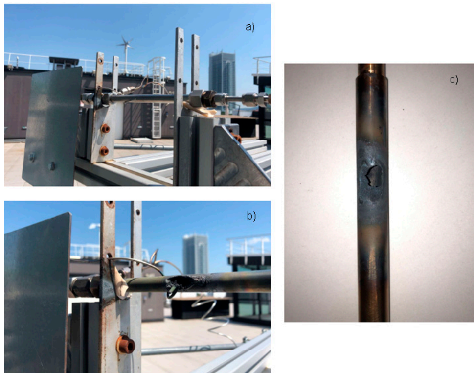
Figure 6. Experimental activity for the metal alloys used (a) Inconel 740H; (b) alloy 625; (c) Haynes 230.
