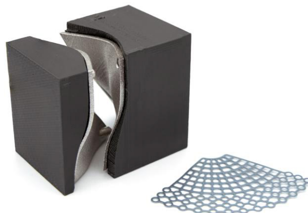
Fig. 8. Preliminary prototypes of the shaping dies.
