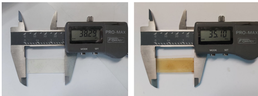
Figure 2. Dimensional and color changes taking place in Base-Zn material after thermal treatment. The left-hand image shows a UV-cured (untreated) sample and the right-hand image shows the same sample after 8 h at 180 °C.
