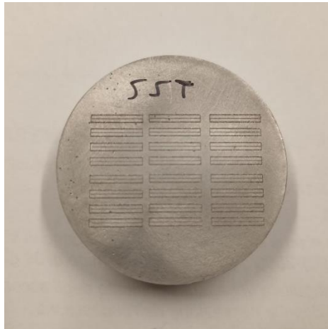
Figure 34: Supporting disk with a diameter of 5 cm with SSTs on the top after printing.
