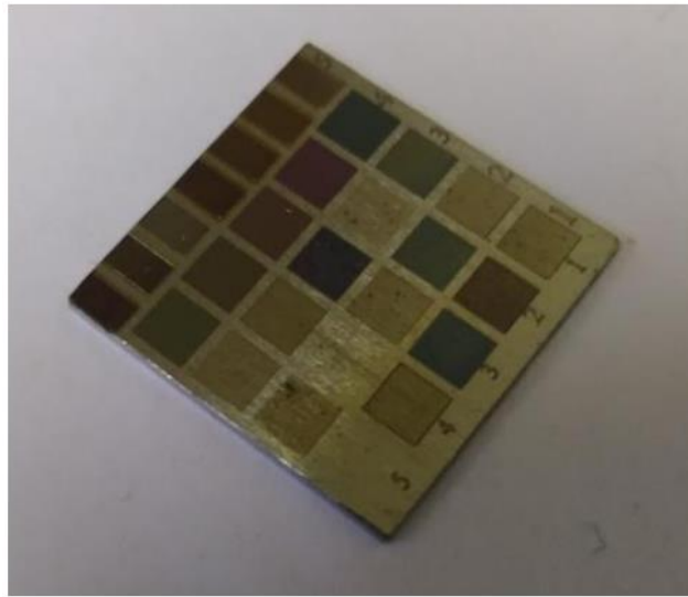
Figure 3.6. Nanosecond laser induced coloration of the crofer sample.
