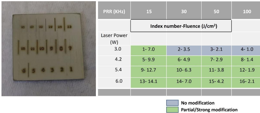
Figure 3.5. Camera image of the single laser scan lines written on the crofer sample using different laser parameters and the corresponding laser parameter table.
