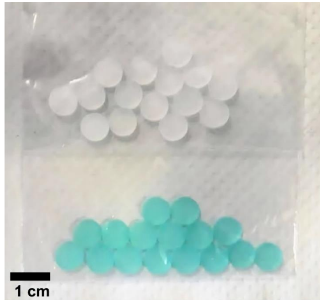
Figure 4.10. Circular disk-shaped samples of undoped (white) and Cu-doped (blue) calcium phosphate glasses, obtained from their corresponding glass rods.
