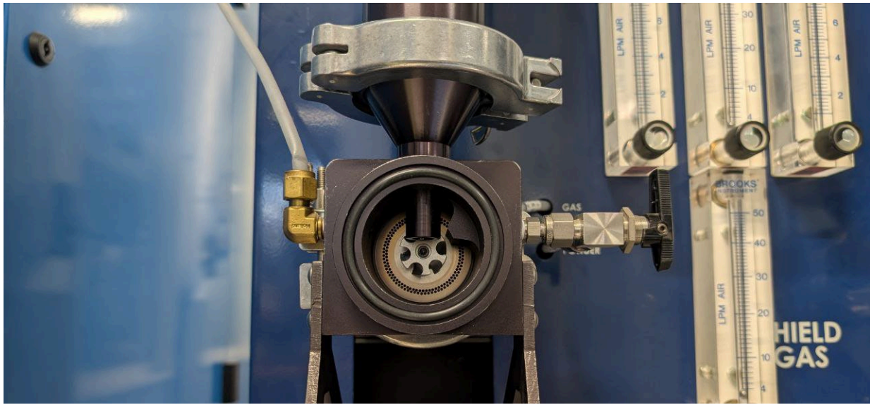
Fig. 1: Optomec CS 150 powder feeder system metering chamber.
