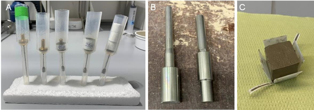
91 92 Fig. 1 Vicat needles for early strength (A), penetrometers (B) and a cube for the 93 compressive strength test (C).
