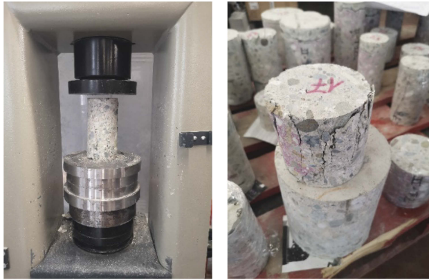
Figure 5. Uni-axial compressive strength tests on concrete samples.
