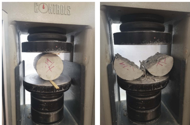
Figure 6. Splitting concrete tensile strength test.
