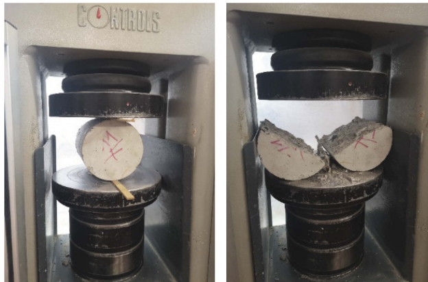
Figure 6. Splitting concrete tensile strength test.
