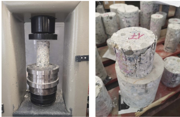
Figure 5. Uni-axial compressive strength tests on concrete samples.
