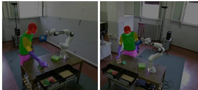
Fig. 1. Example of human-robot collaboration scenario acquired with a multi-view camera setup. Overlaid on each image, the segmentation output of our multi-view human parsing system.
