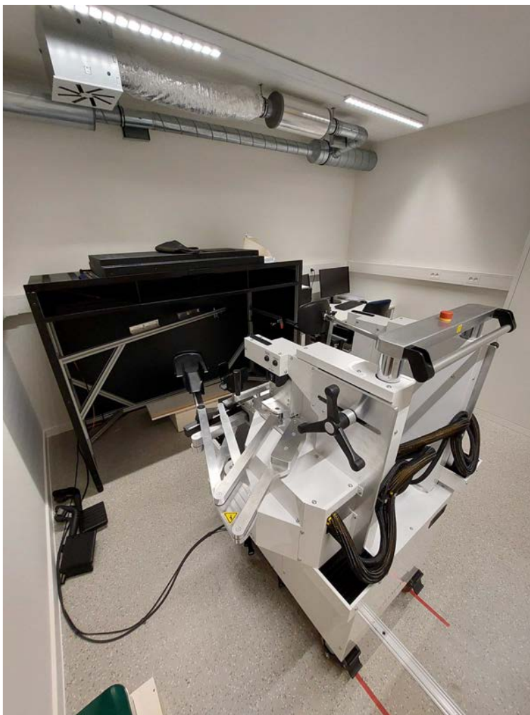
Figure 1: Kinarm Exoskeleton Lab (BKIN Technologies, Kingston, ON, Canada) [20] with integrated EyeLink 1000 Plus system (SR Research, Ottawa, ON, Canada) [21].
