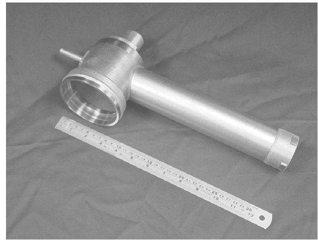
Fig. 31 LP-DED integrated boom/housing [203]
