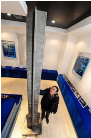
Fig. 21 A 5-m-long titanium wing spar for Comac C919 [190]
