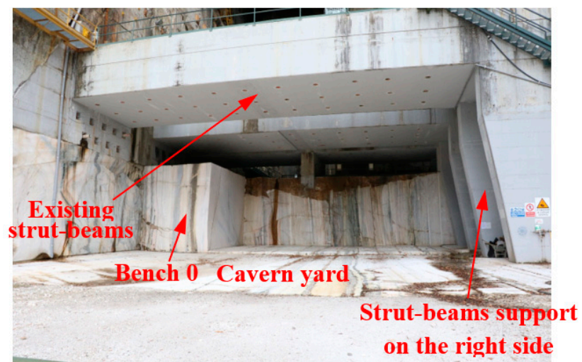
Figure 2. Detail of the first exploitation cut below the beam-struts where the marble extraction works are currently concentrated in the entrance zone of the cavern (Cava Madre of Candoglia).
