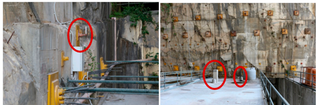
Figure 5. On the left, detail of graduated sights for topographic leveling and wiring for connecting sensors; topographic target inside red oval. On the right, view of the cavern wall with tendons and the suspension terminals of the direct pendulums; measuring points inside red ovals.
