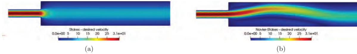
FIGURE 5. Desired velocity profiles : (a) symmetric profile obtained as Stokes solution for \mu = 1 ; (b) asymmetric profile given by the physically stable Navier–Stokes solution for \mu = 0.49 .
