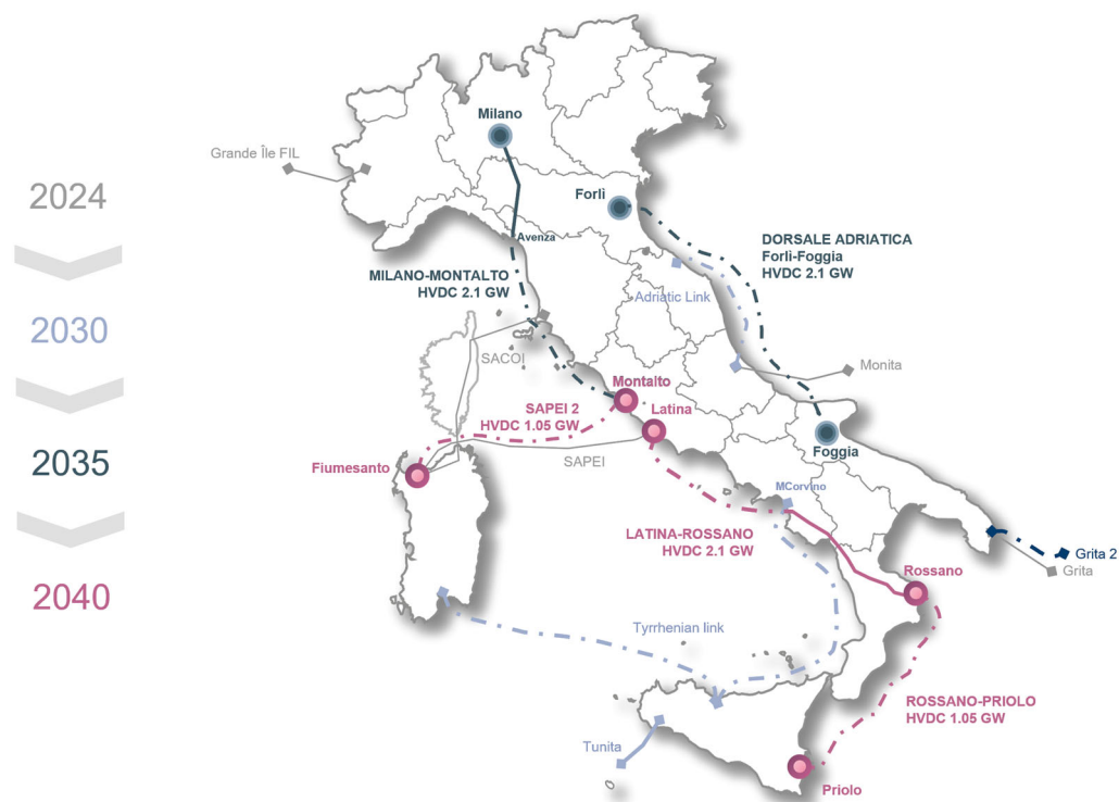
Figure 3. Overview of the HVDC transmission backbones planned within the Hypergrid project. Colour legend: in grey, existing HVDC backbones (2024); in light blue, new ones by 2030; in blue, by 2035; and in fuchsia, by 2040.
