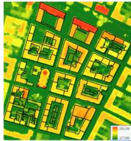
Figure 4: DSM model obtained from the aerial photogrammetry datasets.
