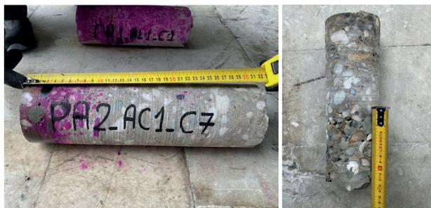
Figure 10 | Sample in the portion of the arch presumably made with Type 680 concrete (on the left), and a sample in the portion of the arch presumably made with Type 500 concrete.
