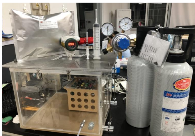
Figure 9. Photo of the air-tight chamber.
