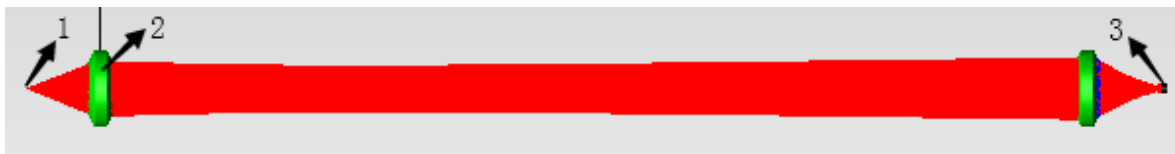
Figure 2. Optical simulation of the two convex lenses, where 1 is the output beam from the paraboloid concentrator, 2 is the convex lens and 3 is the detector.
