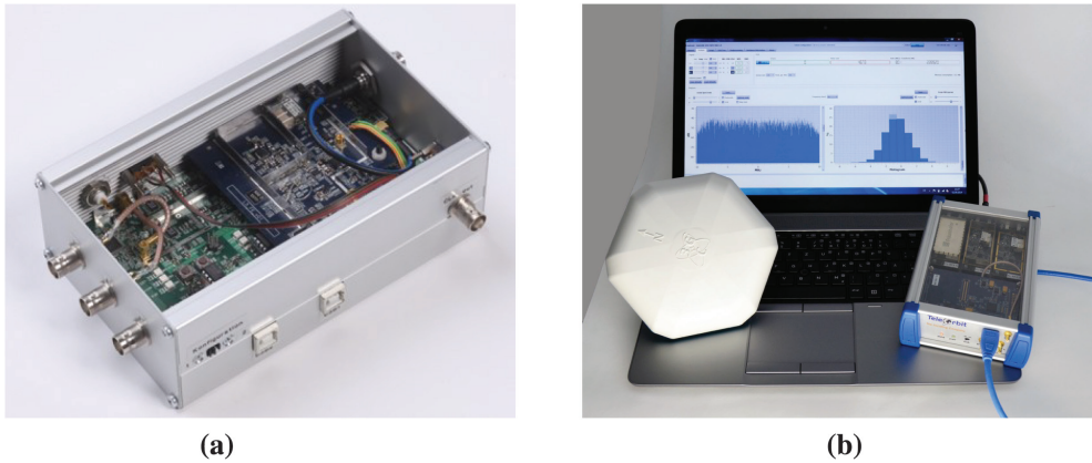
FIGURE 2 Two exemplary USB front-ends from Fraunhofer IIS (a) TriBand USB2.0 front-end from 2006 (b) Flexiband USB3.0 front-end from 2012 onwards
