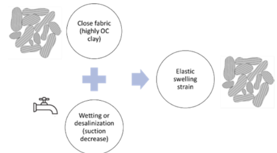
Fig. 2. Schematic of suction reduction effects on clay with closed fabric.
