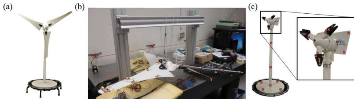
Fig. 47 Schematics of (a) the entire wind turbine [114], (b) bolted blade and hub [115], and (c) the tower structure. Reproduced with permission from Ref. [116], © The Society for Experimental Mechanics, Inc. 2014.
