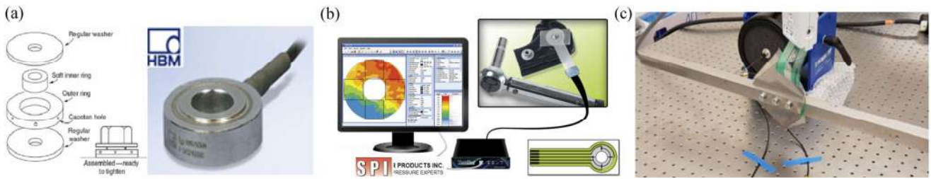
Fig. 8 Measurement techniques, (a) preload indicating washer, (b) pressure indicating washer, and (c) pressure film.
