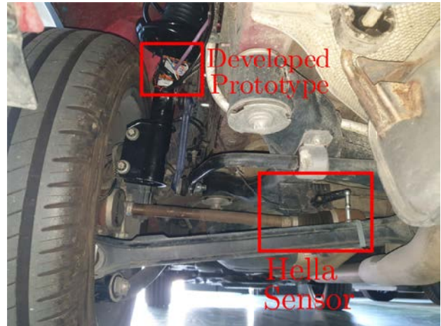
Fig. 15. Democar setting: developed prototype mounted directly on the shock absorber and reference sensor mounted to have a measure proportional to the rod displacement.
