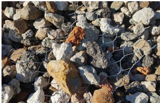
Figure 150 : Recycled aggregates 40-100mm
