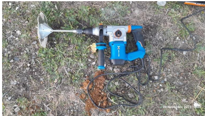
Figure 84 : Pneumatic handcrafted tamper
