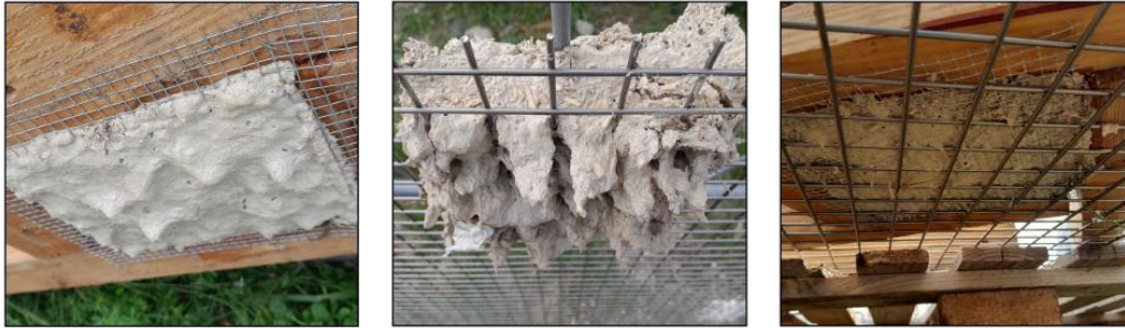
Figure 67 : Behaviour of the mortar in function of its hydration. from left to right : very liquid ; muesli ; paste
