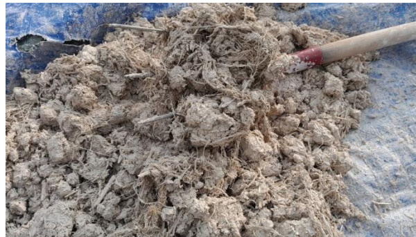
Figure 110 : Hemp-lime mix with long fibres
