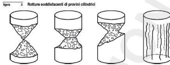
Figure 116 : Failure typologies according to UNI EN 12390
