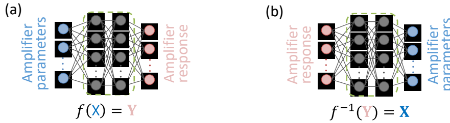
Figure 1 NN models for a fiber amplifier: (a) direct and (b) inverse model.
