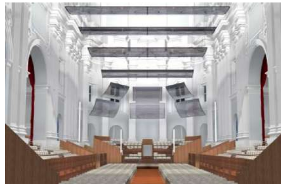
Fig. 9 – Acoustic project design for the adaptation of Santa Lucia's church to an auditorium. Apse side
