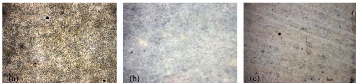
Fig. 8. Surface condition of AAS mortar under 200 freeze-thaw cycles at a 50× magnification. (a) S0, (b) S0.2W0, (c) S0.2W15.
