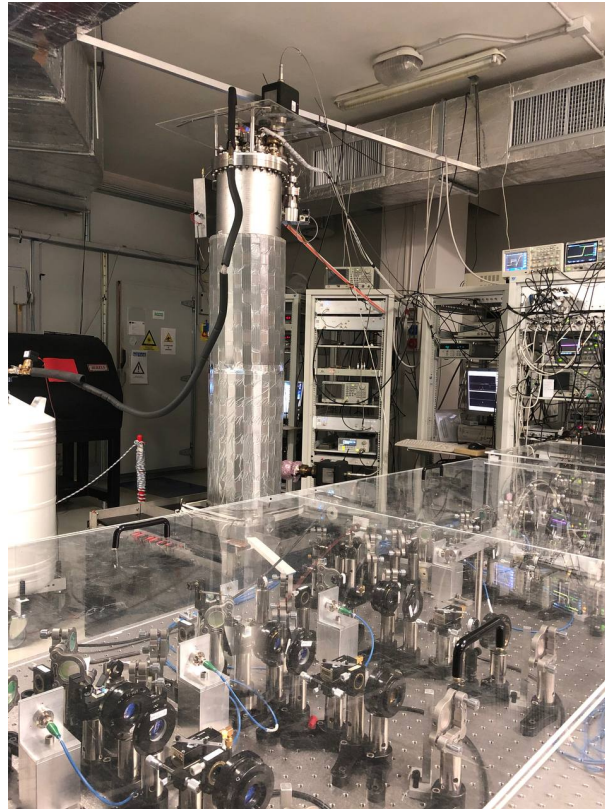
Fig. 4.1 Picture of IT-CsF2: the Italian cryogenic Cs fountain.
