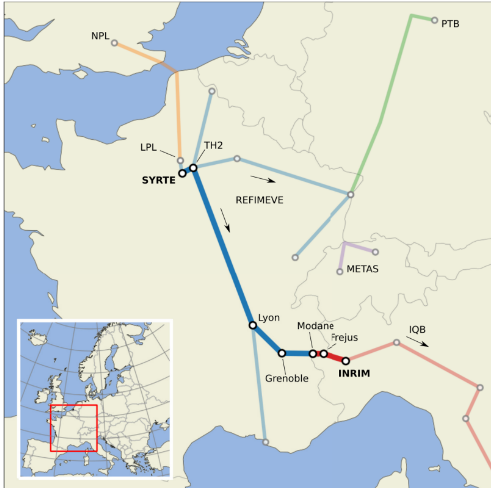
Fig. 4.5 Sketch of the European network of optical fiber links, adapted from [150]. The SYRTE-INTRIM branch is highlighted as a thick line. In blue is illustrated the French REFIMEVE network, while in red is represented the Italian Quantum Backbone (IQB) network. The scheme also shows the branches connecting SYRTE to two other European metrology institutes: NPL in the UK and PTB in Germany, indicated as yellow and green lines, respectively. White empty circles represent intermediate link terminals provided with a repeater laser station (RLS) or a multi-branch laser station (MLS).
