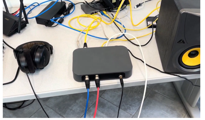
Fig. 1. Embedded NMP device prototype with connected audio and networking interfaces.
