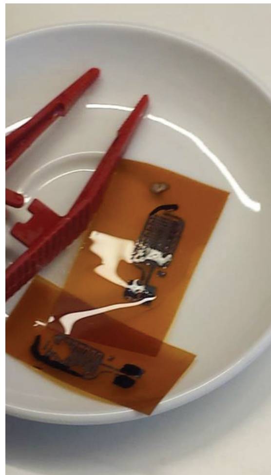
Figure 10. Circuits etched on copper laminated films (Photo: Alvisse Mattozzi)
