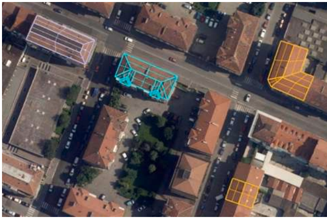
Fig. 7. Roof measurement with gable (orange), hip (cyan), and one gable end/one hip end (purple). (For interpretation of the references to colour in this figure legend, the reader is referred to the web version of this article.) Source: authors' elaboration on top of municipal orthophotos [66].
