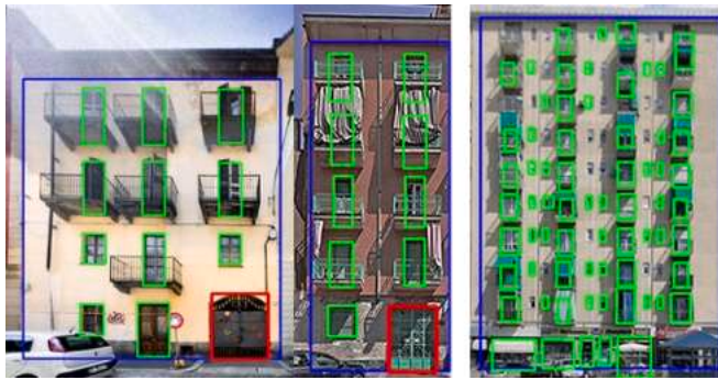
Fig. 4. Detections from the deep learning model with windows (green), wall (blue), and garage door (red). Differences in WWR between detections and ground truth are + 0.1% (left), +3.7% (center), and -6.6% (right). (For interpretation of the references to colour in this figure legend, the reader is referred to the web version of this article.) Source: images are facsimiles of original SVI, using photos taken by authors.
