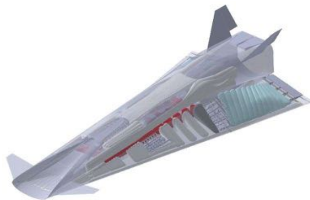
Figure 1. STRATOFly MR3 Vehicle layout with integrated systems.
