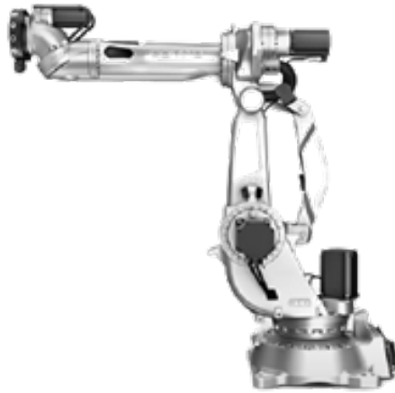
Fig. 8.2 The 6 axis COMAU robotic manipulator NJ4 170 2.5 used for the tests. Image from COMAU website
