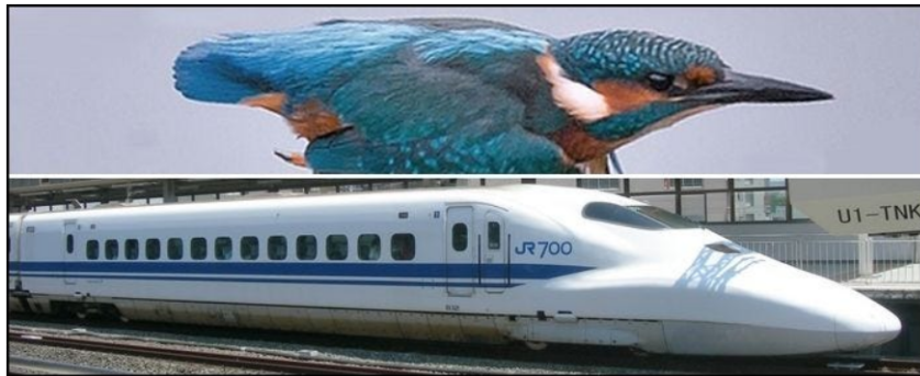
Fig. 6.1 Bullet train nose design compared to a Kingfisher
