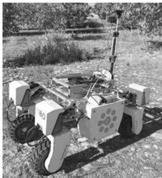
Figure 1. Setup of the ground-based scanning system mounted on Thorvald unmanned ground vehicle.
