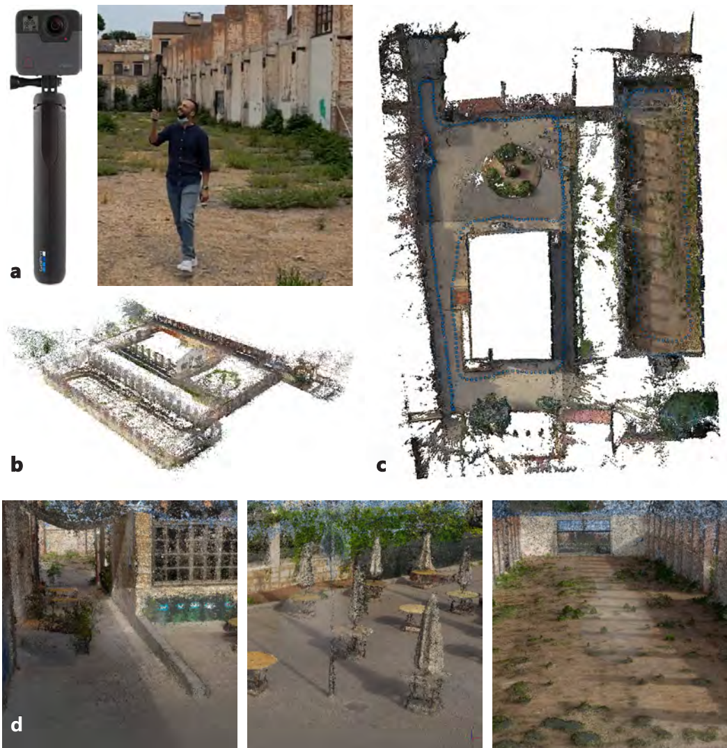
Fig. 3. a) GoPro Fusion 360 and the acquisition on site; b) perspective view of the sparse cloud; c) top view of the dense cloud; d) focuses of the dense cloud.
