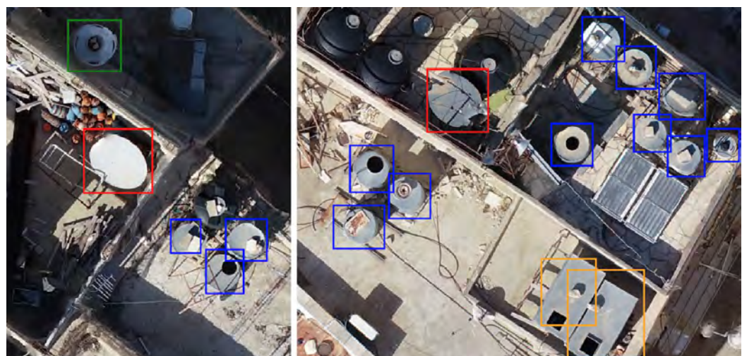
Fig. 4. Figure shows a ortho image with the output of the model overlayed on top. Highlighted examples of Correct Detections, mismatches, competing labels and missed objects. Both images show high precision. Left: False Negative: missed plastic tank close to metallic tanks. Right: False Negative: missed plastic tank. Black tanks area critical due to the shadows on the roofs.
