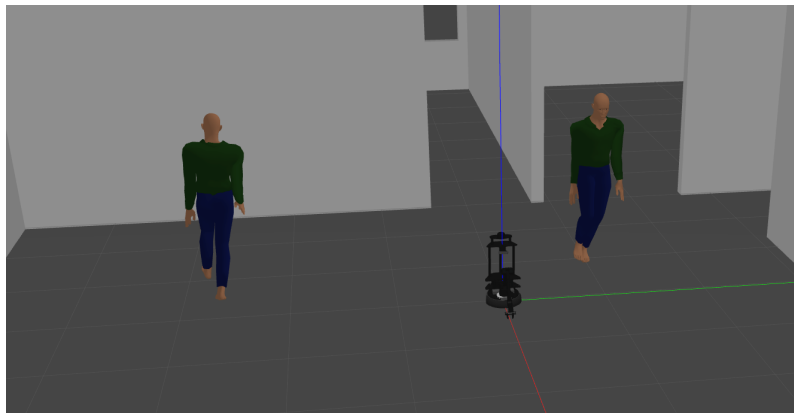
Fig. 5.12 A scenario with a robot and two pedestrians simulated using the SFM plugin within the Gazebo environment.
