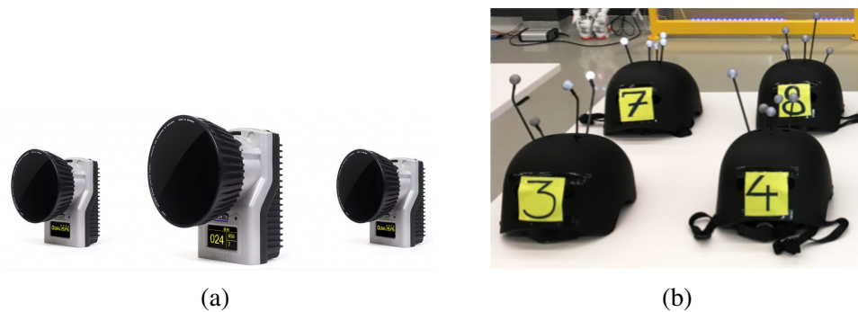
Fig. 5.4 (a) Qualisys Oqus 7+ infrared cameras; (b) Helmets equipped with reflective markers, designed for pedestrian tracking.
