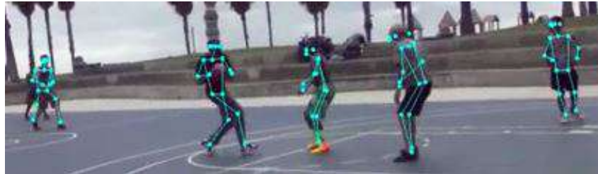
Fig. 6.8 An example of the body tracking mode of Zed2 [6].
