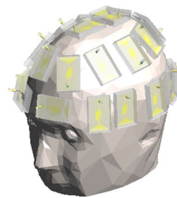
Fig. 1. MWI system: antennas' array with a helmet configuration.
