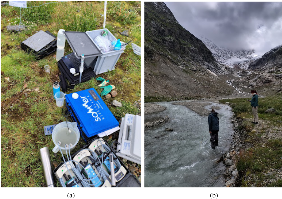
Fig. 4.3. (a) Material used during the discharge measuring campaign at SteinGletscher; (b) Measurement of river velocity.
