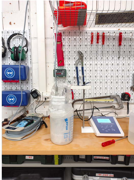
Fig. 4.4. Lab set up to keep the cylinder with river water cool.
