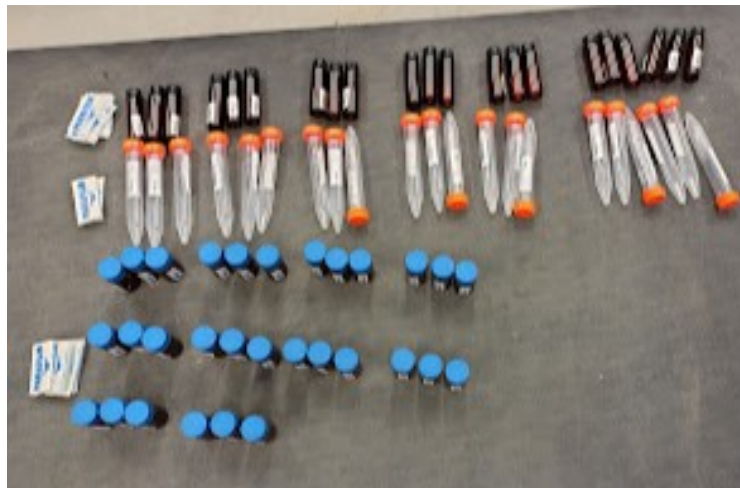
Fig. 4.9. Prepared vials (from top to bottom): brown glass vials for snow sampling, orange-cap plastic vials for snow sampling, blue-cap glass vials for ice sampling.
