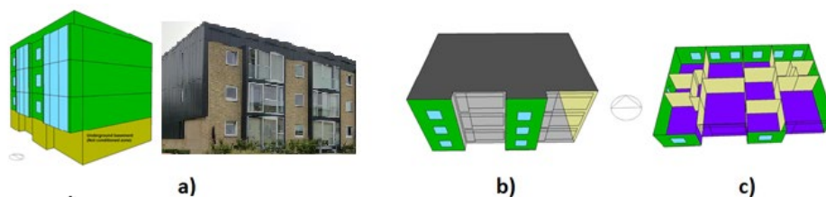
Figure 1. From left: a) Building from the outside, b) mono-zone model – one staircase as thermal zone, c) multi-zone model – each room as a thermal zone.
