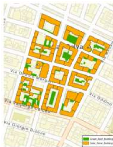
Figure 6 Buildings suitable for Solar panel installation (yellow) and Green Roofs (green) based on orientation and available rooftop area criteria.
