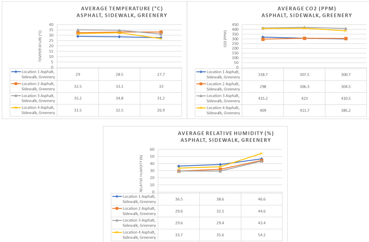
Fig. 4. The average values per each location including all types of pavements. (Authors' elaboration.)
