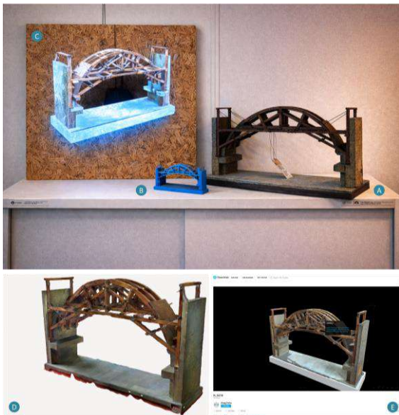
Figure 8: Example of a model of a complete suit of armour, known as suspended armour, with wooden fittings ( Modello di una armatura completa, detta sospesa con ferramenta in legno ), 40x76x20 cm, Inv. 47 (1865-1887, DISEG); A –original wooden model; B - 3D printed model; C – holographic model; D – polycam model; E – sketchfab model).
