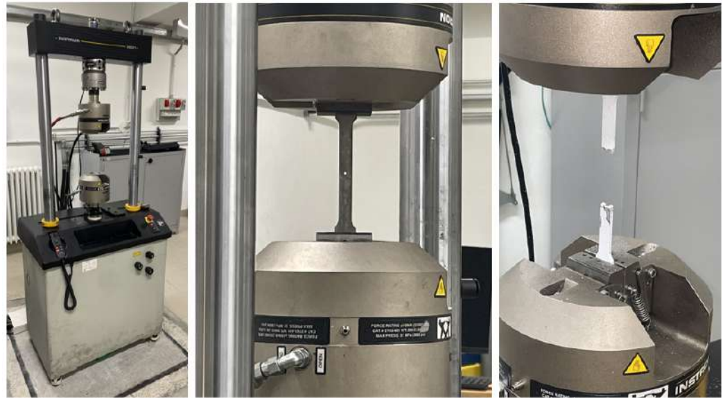
Figure 4. Specimen installed in the fatigue test machine.
