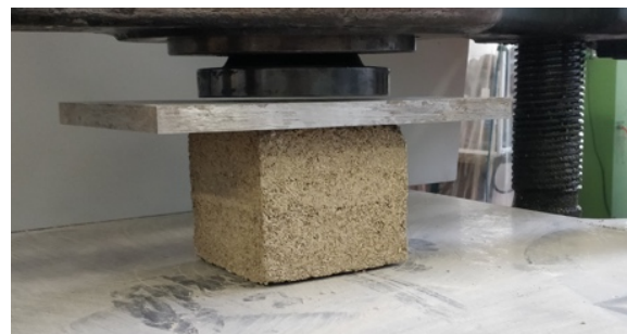
Figure 12: Compression tests of brick and cube samples
