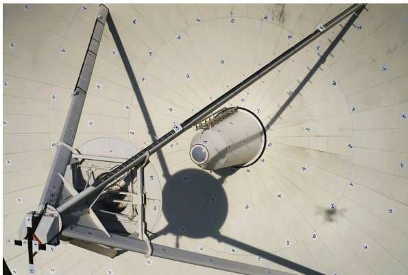
Fig. 3 Coded targets on the telescope (main and subreflector as well on struts and tube in the center)
