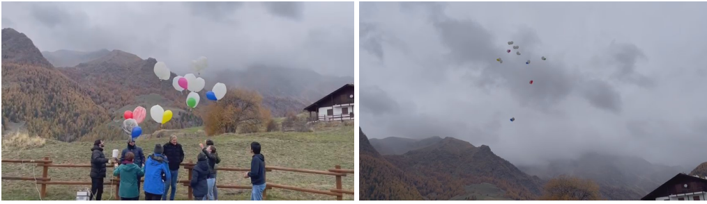
Figure 5.6: Release of a cluster of 10 radiosondes into alpine atmosphere for free floating during OAVdA experiment, November 3, 2022.
