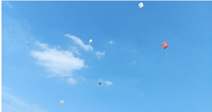
Figure 4.16: Experiment with five tethered radiosondes at INRIM on September 29, 2021. Two radiosondes tracked using video camera were marked in red and black.
