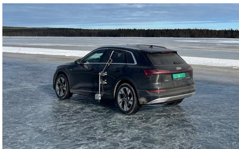
Figure 1. The case study Audi e-tron at the Ebbenjarka testing facility (Sweden), including the Kistler Correvit S-350 sensor, providing accurate measurements of the velocity components.
